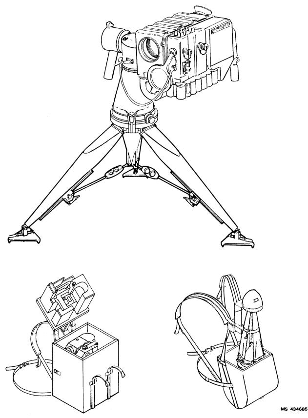
Electro-Optical Target Designator Set. AN/TVQ-2 (G/VLLD)
