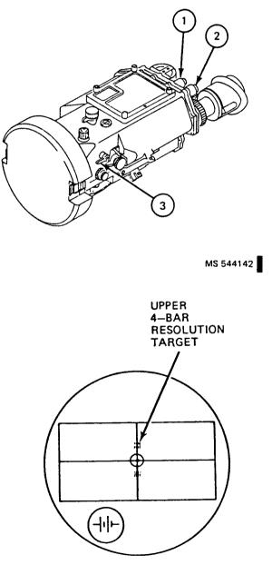
BORESIGHT CORRECTLY ALIGNED (WFOV)
