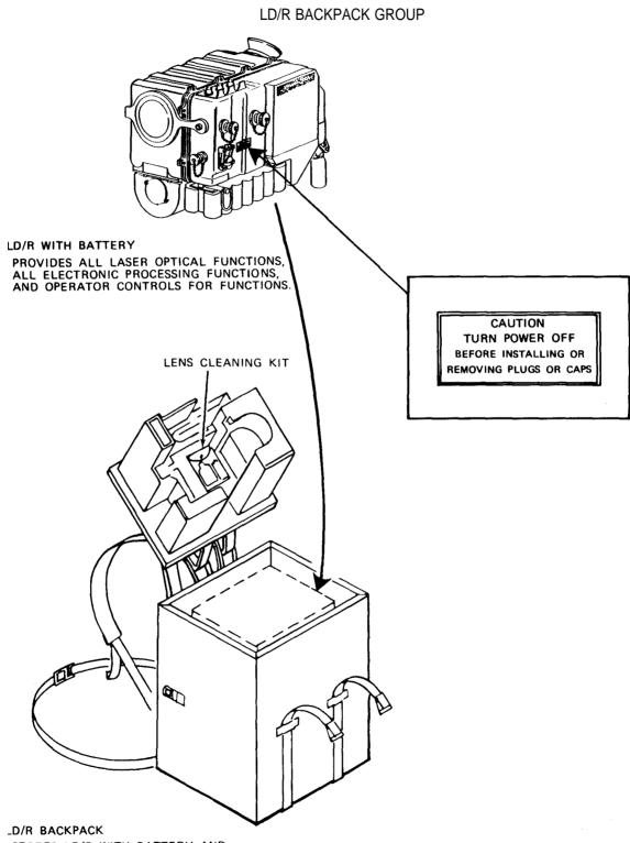
STORES LD/R WITH BATTERY AND LENS CLEANING KIT FOR TRANSPORT.
