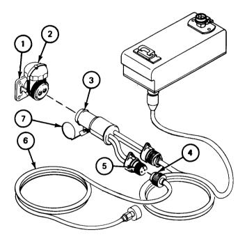
3.1. REMOVE AND PACK EMI FILTER, NATO CONNECTOR, SLAVE CABLE, AND VEHICLE POWER CABLE (CONT)
