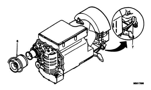
6. Remove front lens cover (6) from nightsight. Place nightsight latching handle (9) in the rear position (toward eyepiece), and mount nightsight on top of platform (13). Make sure platform cam post (14) lines up with nightsight cam opening (10) and V-ways (11 and 12) on bottom of nightsight line up with V-ways (15 and 16) on top of platform. It may be 'necessary to slightly rotate nightsight to get a good fit.
