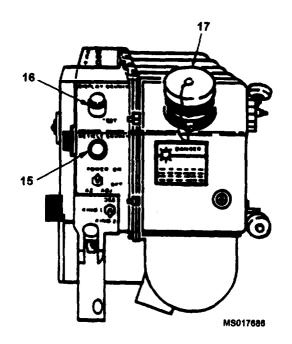
Rotate DISPLAY BRIGHT control (16) fully cw; but DO NOT place in TEST (detent) position.
